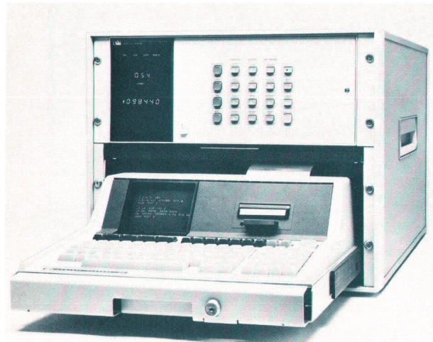
Fig. 1. The 3054DL system combines a 3497A Data Acquisition/Control Unit with various accessories and an HP-85 as the controller in a packaged arrangement for easy and convenient data logging. The system comes with extensive software for displaying and analyzing data, thermocouple voltage-to-temperature conversions, and configuring data logging setups.
