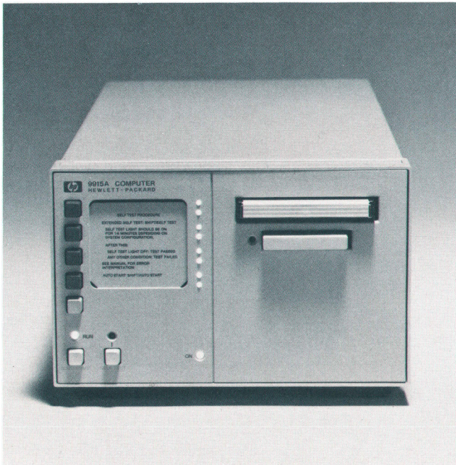
Fig. 1. The HP Model 9915A Modular Computer is a powerful desktop computer in a rack-mountable package designed for industrial environments. This low-cost computer is easy to use for measurement automation.
